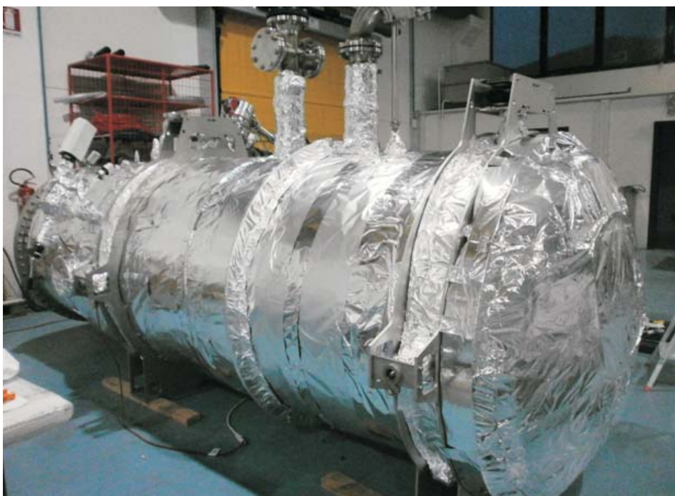
Figure: The first cryolink at Alca Company in Schio (Vicenza), ready for bake-out test
